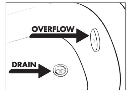
If the above steps do not unclog your drain, Bath Fitter recommends another low cost natural solution. Remove stopper pour equal parts baking soda and white vinegar into the drain. Next pour hot water into the drain. Re-install the pop-up stopper.
